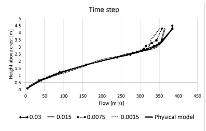
Figure 7a. Rating curves from parameter sensitivity tests: time step. Situation without air and smooth walls.
