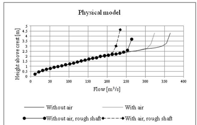
Figure 4: Stage-discharge curves from the physical model test
