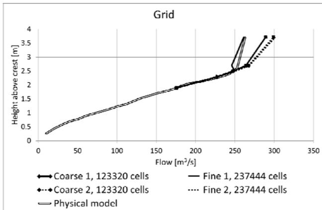
Figure 7c. Rating curves from parameter sensitivity tests: grid size. Situation without air and rough walls.
