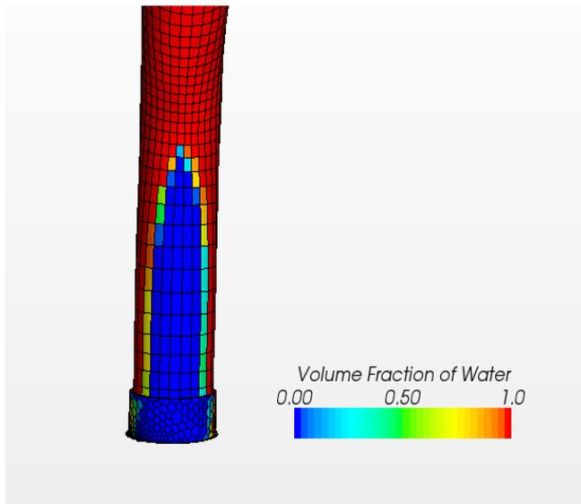
Figure 8 a. Air concentrations at the vertical pipe outlet for situation without air and smooth walls.
