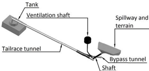
Figure 2. 3D sketch of the spillway system as built in the laboratory.
