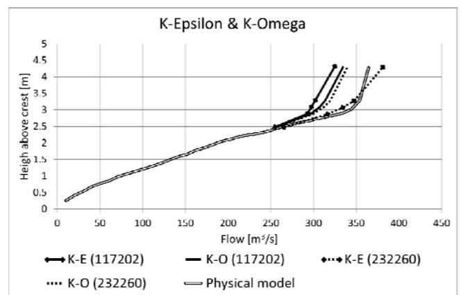
Figure 7b. Rating curves from parameter sensitivity tests: turbulence model. Situation without air and smooth walls.
