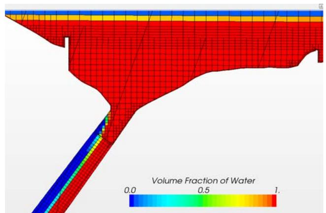
Figure 8 c. Air concentration at the top of the 45 degree shaft for situation with air and smooth walls.
