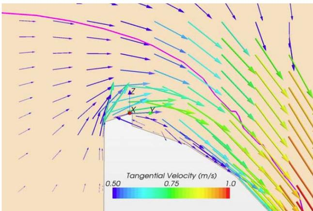
Figure 6. Velocity vectors over the spillway. The pink line shows the water level.
