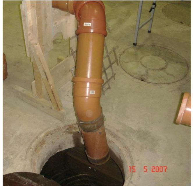
Figure 3. PVC pipe at the end of the tunnel in the laboratory model (Røneid & Sæter, 2007)
