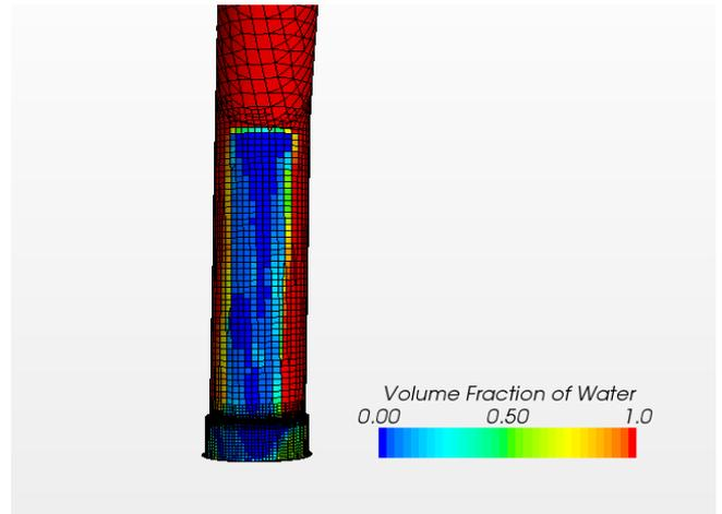
Figure 8 b. Air concentrations at the vertical pipe outlet for situation without air and smooth walls.
