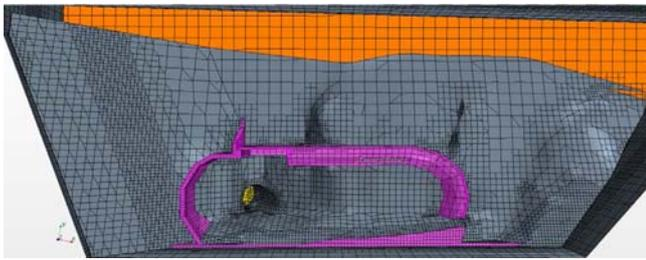
Figure 5. Trimmed grid of the reservoir and spillway seen from above. The concrete construction is shown with pink color. The yellow area is the 45 degree shaft. The orange area is the inlet of the model.
