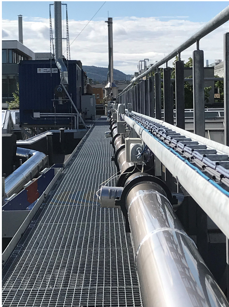
Figure 2: The ECCSEL depressurization tube. The CO 2 is vented through the stack in the background. The container at the left contains support equipment.
