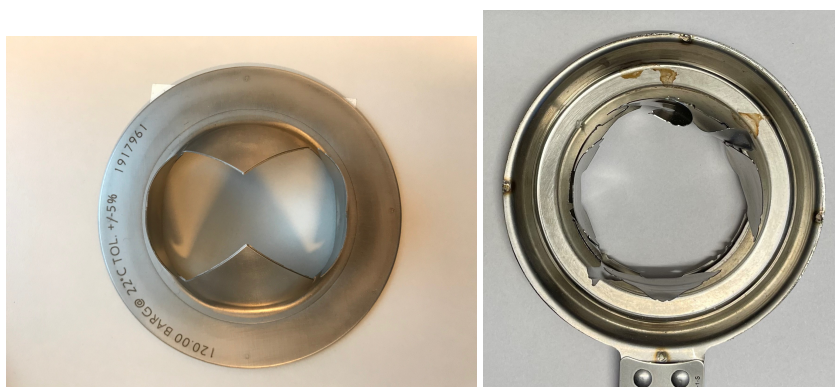
(a) X-scored rupture disk after test.
